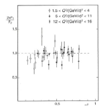
Along y-axis  $\frac{2xF_1}{F_2}$  is plotted and it is seen that it is around 1. Hence electrons are scatted by spin  $\frac{1}{2}$  quarks. The value would have been 0 if electrons get scattered by spin 0 structureless particles.
