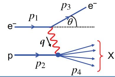
Due to the finite proton size, elastic scattering at high  $q^2$  is unlikely and inelastic reactions where the proton breaks up dominate.
